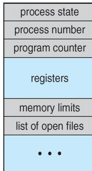
Figure 3.3 Process control block (PCB)
